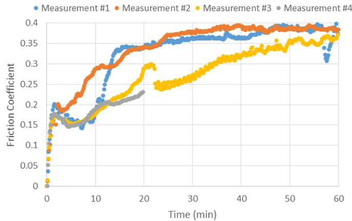
Figure 8: Measurements of the water lubricity using the dynamic lubricity tester.
