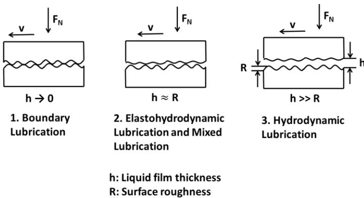
Figure 2: Illustration of different lubrication regions (modified from Hironaka, 1984).
