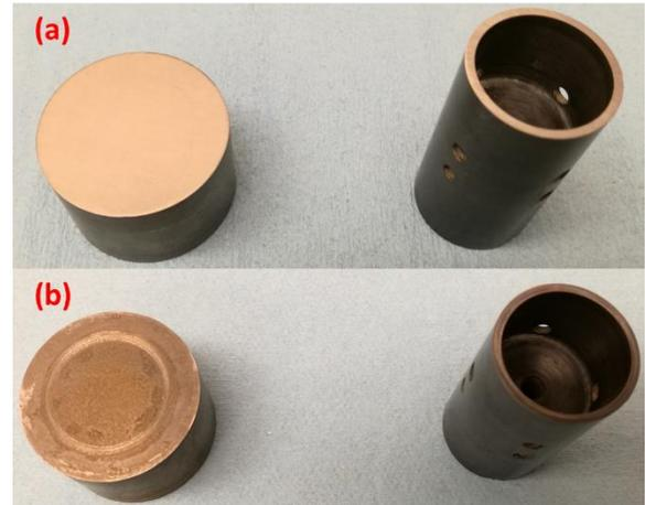
Figure 6: Metal block and rubbing shoe (a) before and (b) after a lubricity test.
