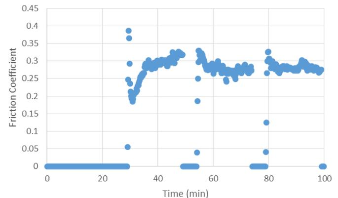
Figure 10: Friction coefficient of the base WBM with no lubricant on an Alabama marble core.
