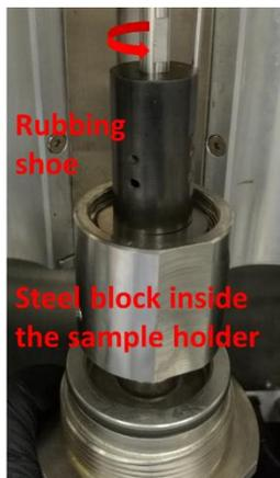
Figure 5: Configuration of the rubbing shoe and steel block inside the sample cell.
