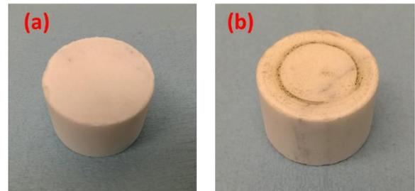
Figure 7: Alabama marble core (a) before and (b) after a lubricity test.
