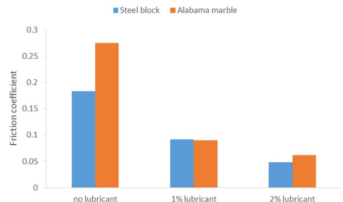
Figure 11: Friction coefficient of the WBM with and without lubricant when steel block and Alabama marble core were used in the lubricity measurement.
