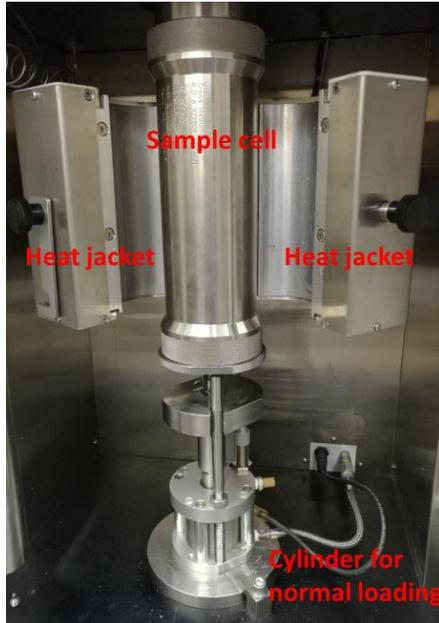
Figure 4: Dynamic lubricity tester.
