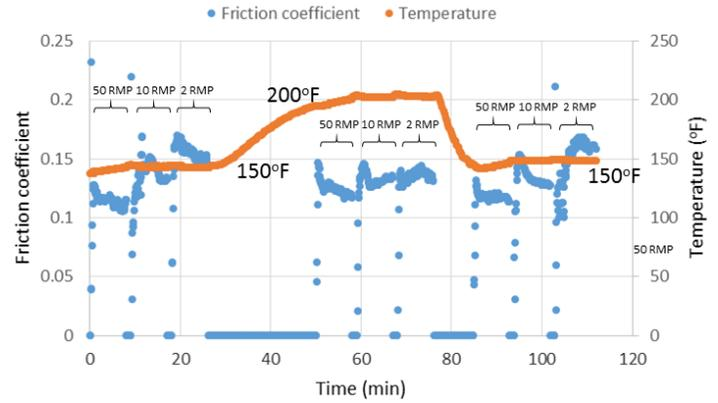
Figure 9: Measurements of the lubricity of a base oil using the dynamic lubricity tester.
