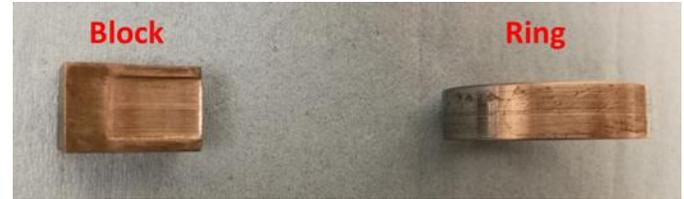
Figure 3: Ring and block used in the traditional EP/lubricity tester.
