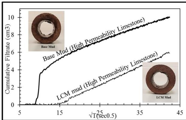
Figure 7: Dynamic filtration pattern in 70mD Limestone
