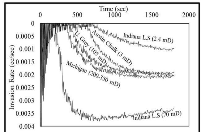
Figure 11: LCM mud dynamic filtrate invasion rates
