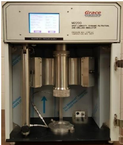
Figure 3: Dynamic-radial filtration set up
