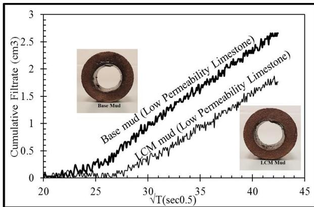
Figure 6: Dynamic filtration pattern in 2.4mD Limestone
