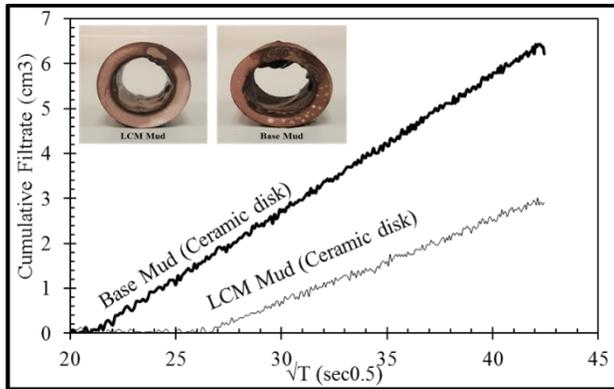
Figure 9: Dynamic filtration in 5µm Ceramic Disk
